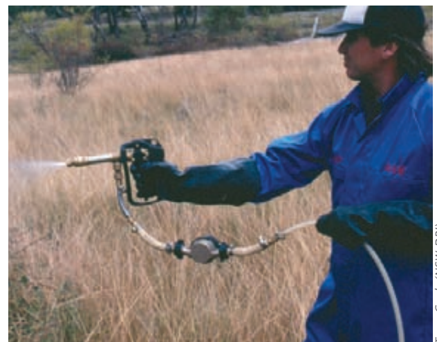
Hand gun with a flow meter (note that PPE is not being used because the operator is only spraying water as a demonstration).
