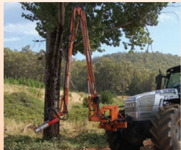
The Spraying Mantis mounted on a tractor.
